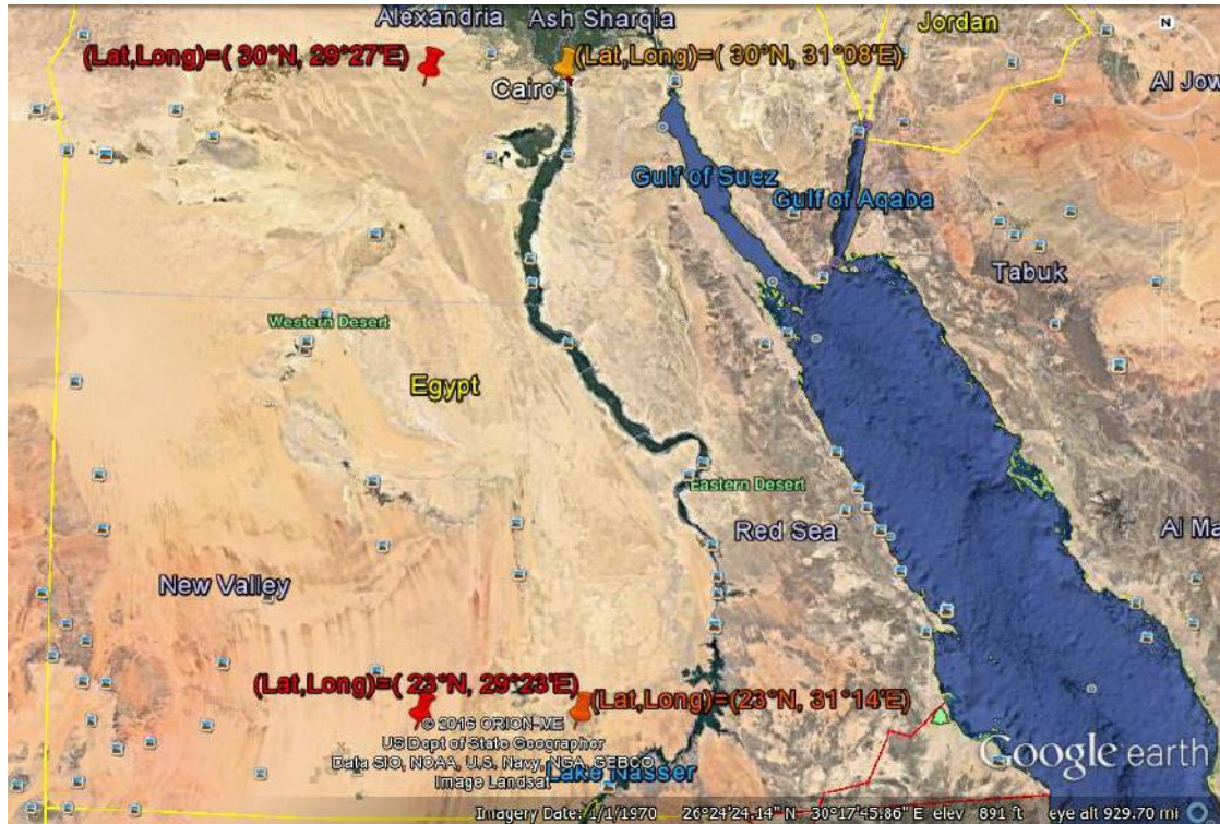
Figure 8: Locations when ETM and UTM Scale Factors are equal for Red Belt Zone in Egypt.
